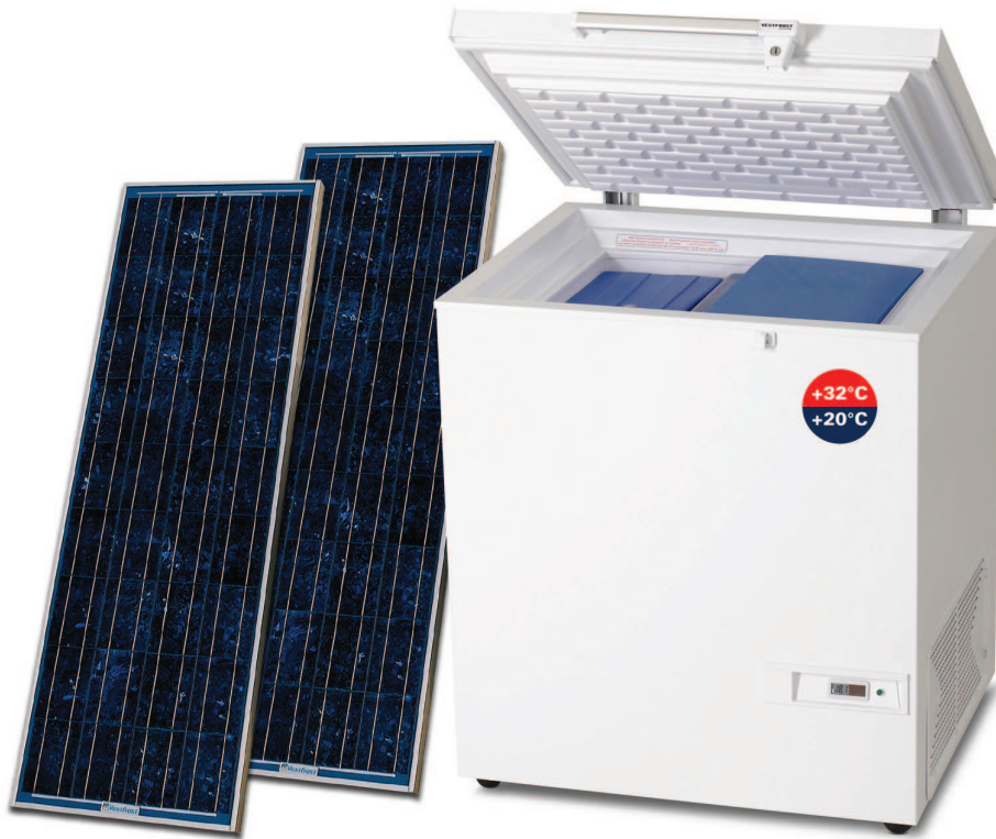
Photo 4: Photo of the SolarChill vaccine refrigerator, produced by Vestfrost. The refrigerant is R600a (isobutane). Ice storage ensures cooling during night-time.
